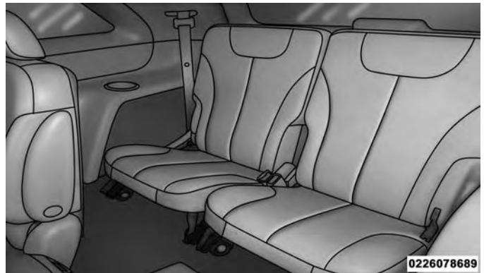
3rd Row Seat Has No LATCH Lower Anchorages (2004–2008 Model Years)
