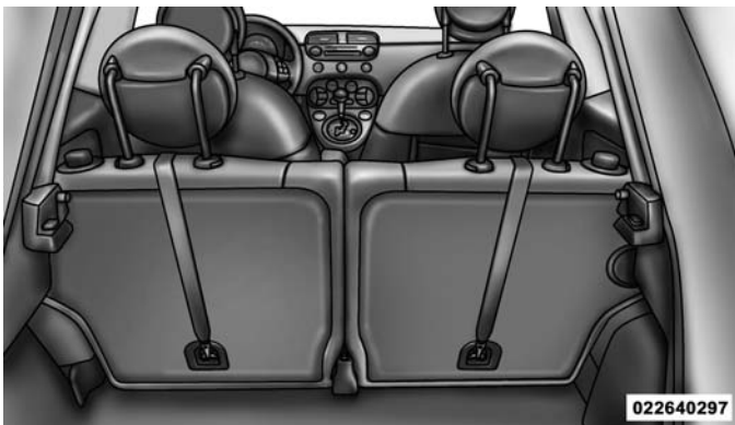
Rear Seat Tether Strap Mounting
