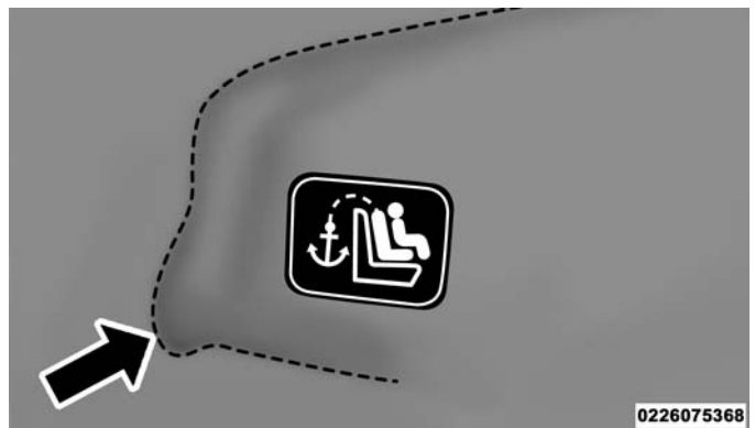
Child Tether Anchor Location (2001–2006 Model Years)
