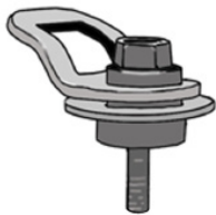
Pre-assembled tether anchor for installation into a weld nut. Anchor hardware is made up of the bolt, bracket, and spacer.
