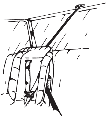
Station wagon, hatchback: tether anchored in the top of the rear door frame
