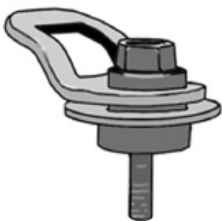
Pre-assembled tether anchor for installation into a weld nut. This is screwed in to the stated tightness. Make sure not to force it into a welded nut.
